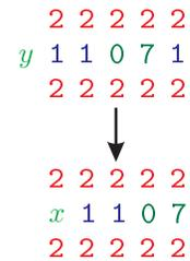
Figure 1: A data-path. The data signal '7 0' travels along the data-path. The state of cell  $x$  in the updated state is dependent on the state of cell  $y$ . If  $y = 1$ , then in the updated state  $x = 1$ .
