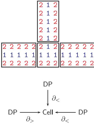
Figure 3: A T-connection. The image at the top shows a T-connection as realised in a cellular automaton; the diagram below describes the same connectivity in the schematic form described in the following subsection.
